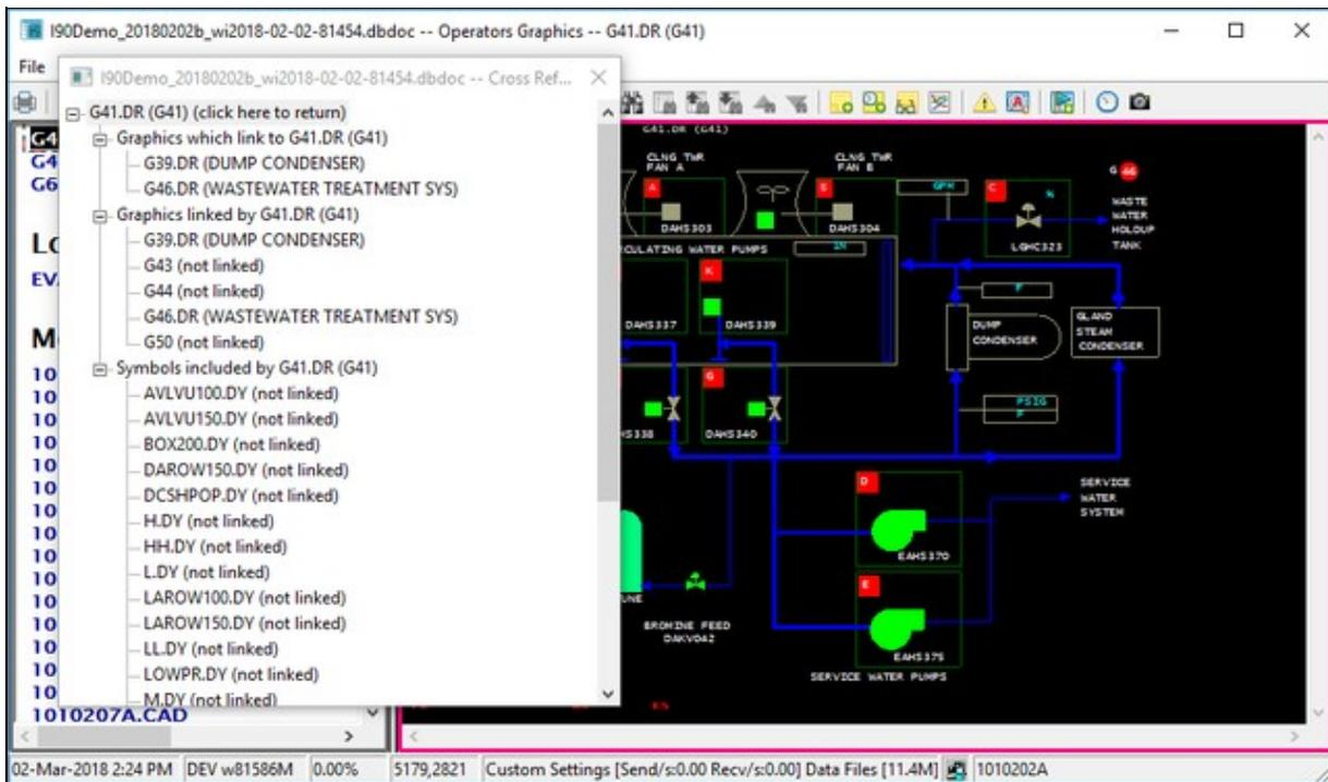
A separate floating window will be opened showing you the different Graphics Cross References categories, handily displayed in a tree view:
