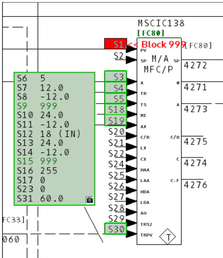
Live specs can then be turned on and off individually for each block by double clicking the camera in the bottom right corner.
