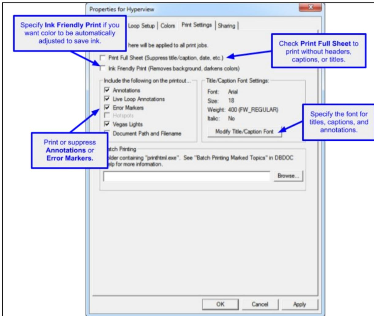
Any setting changes made here in the print dialog under the **Advanced Options** (e.g. **Suppress automatic color reversal**, **Annotations**, etc.) will be reflected in the **Print Settings** tab under **Options**.
